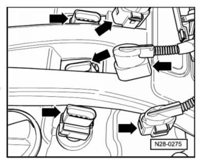
Fit connectors 1...6 for ignition coils with output stages.
